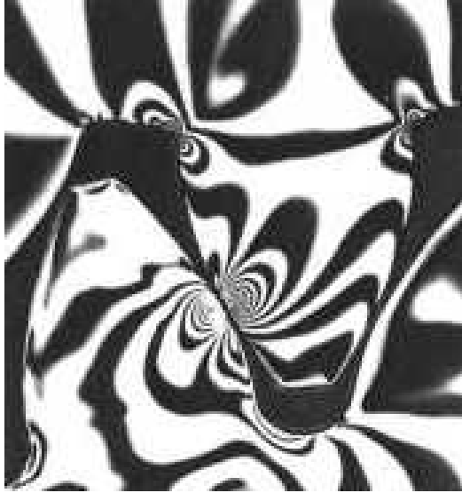
Photoelastic pattern of stresses in a spur gear tooth
